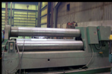
8'-0" Plate Rolls Capacity 1 1/4"
